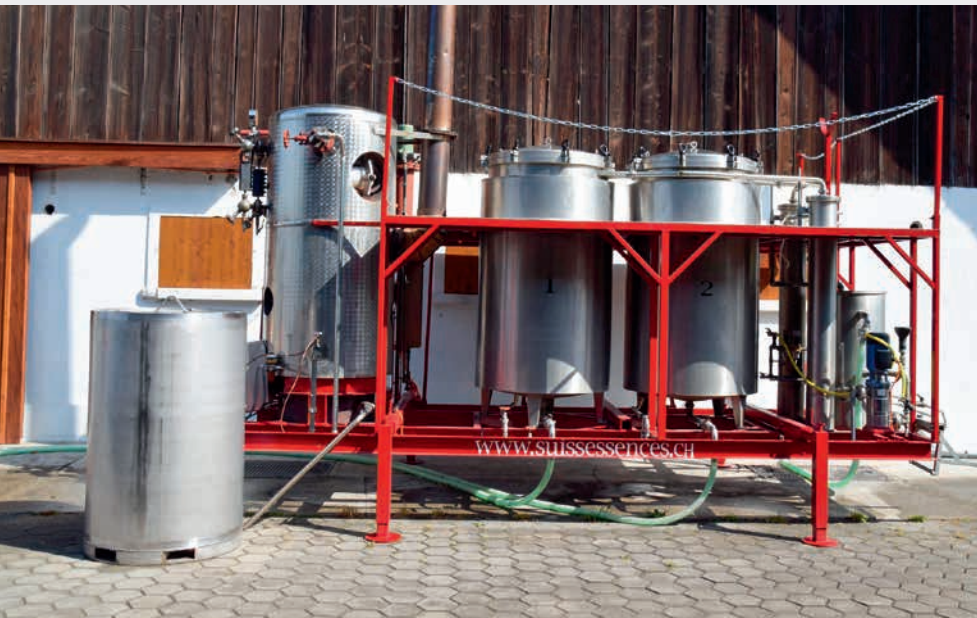
Essential oils are extracted by steam distillation. Guided tours are available for groups of 15 or more.
